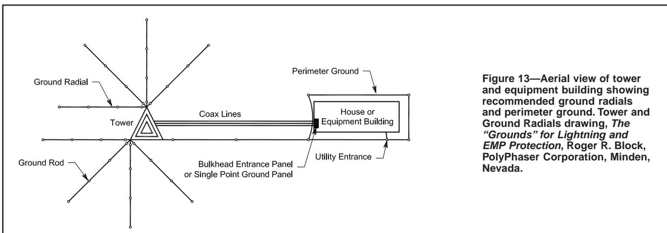
Figure 13—Aerial view of tower and equipment building showing recommended ground radials and perimeter ground. Tower and Ground Radials drawing, *The "Grounds" for Lightning and EMP Protection*, Roger R. Block, PolyPhaser Corporation, Minden, Nevada.
