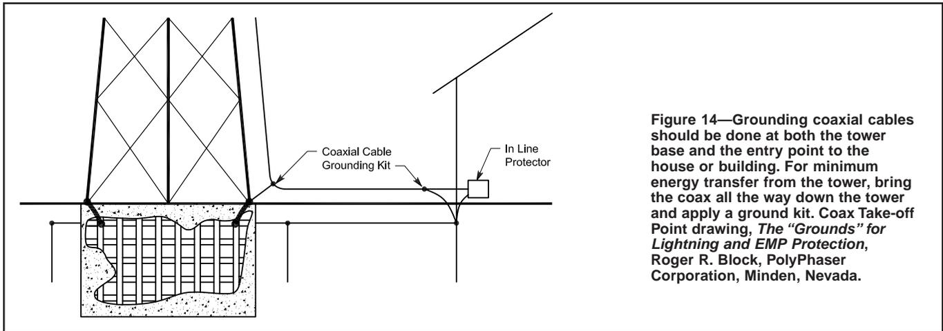
**Figure 14—Grounding coaxial cables should be done at both the tower base and the entry point to the house or building. For minimum energy transfer from the tower, bring the coax all the way down the tower and apply a ground kit. Coax Take-off Point drawing, *The “Grounds” for Lightning and EMP Protection*, Roger R. Block, PolyPhaser Corporation, Minden, Nevada.**
