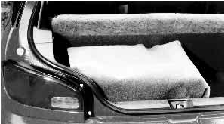
Figure 24 — Neutral-colored material keeps the 500-watt installation out of sight in the GEO Metro
