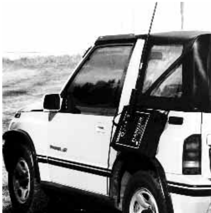
Figure 13 — Suction cups can adhere to the body of the GEO Tracker. The straps maintain pressure on suc- tion cups.
