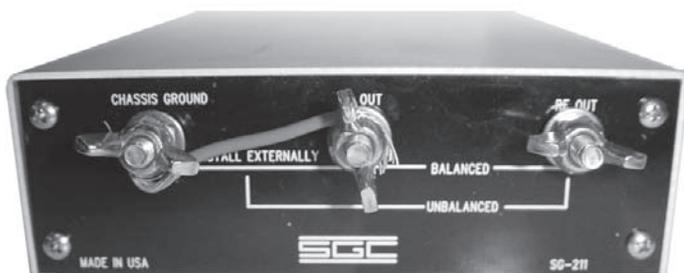
A wide variety of antennas can be connected to the SG-211. A set of wing nuts for connecting balanced or unbalanced antennas is provided on the back panel.
