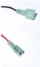
A black wire and a red wire are provided without connectors for 12 VDC power. The red wire should be connected to 12 VDC and the black wire to ground. The speaker unit should operate well with voltages from 10-15 volts. The unit itself is protected against power reversal, so there will be no harm if it is connected backwards inadvertently.
